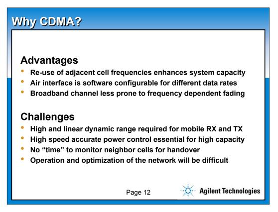
CDMA technology offers a number of advantages over conventional FDMA and TDMA access technologies, however these advantages do not come for free. The basic complexity of layer 1 in CDMA is very high, although once the initial design has been integrated into high-volume ASICs, the costs will come down.
