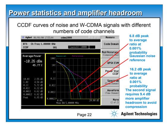
This slide shows a measurement of the Complimentary Cumulative Distribution Function (CCDF) for three different signals. This measure shows, on a log/log scale, the percentage of the time the signal spends above the long term average power. This is also known as the "peak to average ratio" and, for W-CDMA where the baseband signal statistics vary with loading, should always be quoted in conjunction with a probability.
