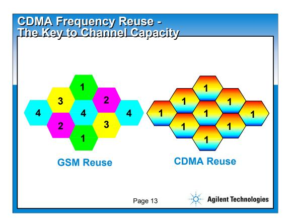
The capacity advantage of CDMA is realized by many technical innovations. One of the most important is the reuse of the same frequency in every sector of every cell. In IS-136 and analog cellular systems, there is a 7 cell repeat factor, with 3 sectors. This means that only one out of every 21 channels is available to each sector. GSM usually uses a repeat of 4, with 3 sectors, for a reuse of one out of twelve.
