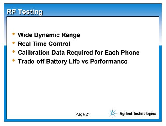
There are several key differences between CDMA technologies and analog or other TDMA technologies. One of the biggest differences is the transmit dynamic range requirement. GSM phones operate over no more than 40 dB transmit power range. CDMA phones have to operate over a much wider range, up to about 80 dB. In addition, there are design specs on the accuracy of this level, as well as the accuracy of the phone to measure the receive level over this entire range.
