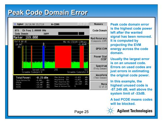
Peak Code Domain Error (PCDE) is an important measure of modulation quality in W-CDMA. The PCDE is the largest measurable code power due to modulation error. In the above example, the eight used codes are clearly visible, and all other codes are seen as noise. The maximum inactive channel power is - 54.249 dB at a factor of 512 which is well above the system specification of -33 dB at a spreading factor of 256.
